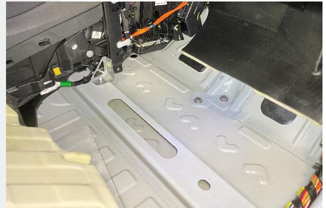
✗ Figure 7 – Butyl patch missing on RH side
