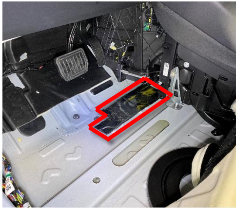
✓ Figure 4 – Butyl patch installed on LH side
