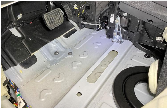
✗ Figure 6 – Butyl patch missing on LH side
